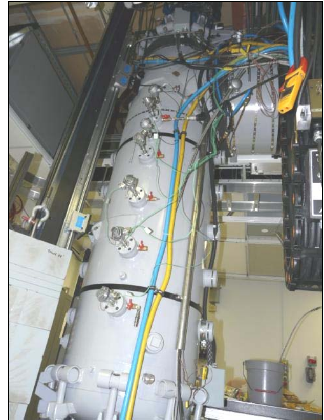
Pressurized entrained flow reactor
